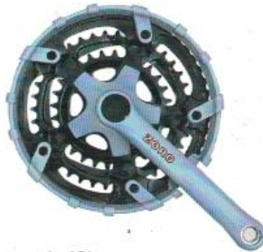
DO - 351 TRIPPLE CHAINWHEEL & CRANK Index Type cotterless 170mm Black powder coated with rounded PVC Guard & Crank PVC Moulded Black/ Gray Teeth 28-38-48 / 24-34-42 for Chain : 1/2" x 3/32"
