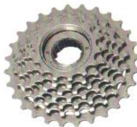
DO - 317 7 Multi Speed Freewheel Non Index type Teeth = 14 to 28 / 32 Chain 1/2" x 3/32" Thread 34.80 x 24 TPI, Golden, Black Colour
