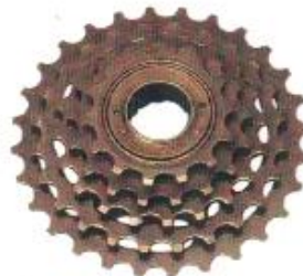
DO - 316 5 Multi Speed Freewheel Teeth = 14 to 22 or 14 to 28 Chain 1/2" x 3/32" Thread 34.80 x 24 TPI, Golden / Black Colour
