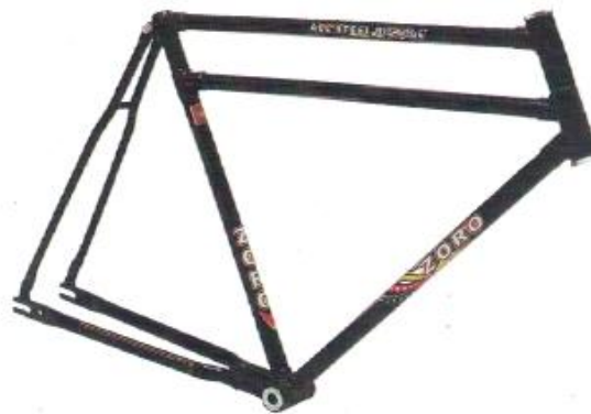
DO - 155 Raleigh Type Double Bar Brazed up Lugs & Shell Available size : 22" / 24"
