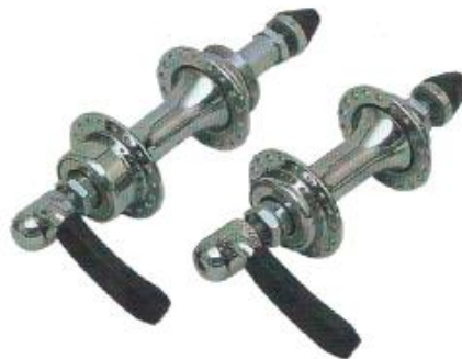
DO - 535 HUB Conical Quick Release Axle Rear 136 / 138 mm with spacer Front 102 / 108 / 110 mm
