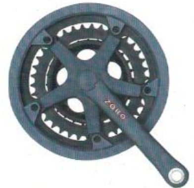
DO - 346 TRIPPLE CHAINWHEEL & CRANK cotterless 170 mm Black powder coated with PVC Guard & Crank PVC Moulded Black / Gray Teeth = 28 - 38 - 48 / 24 - 34 - 42 For Chain = 1/2" x 3/32"
