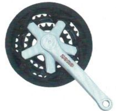
DO - 349 TRIPPLE CHAINWHEEL & BENT CRANK cotterless 170 mm powder coated with PVC Guard & Crank PVC Coated Black / Gray / White Teeth = 28 - 38 - 48 / 24 - 34 - 42 For Chain = 1/2" x 3/32"
