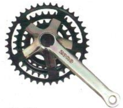
DO - 352 TRIPPLE CHAINWHEEL & CRANK cotterless 170 mm Black powder coated without Guard Crank PVC Moulded Black / Gray Teeth = 28 - 38 - 48 / 24 - 34 - 42 For Chain = 1/2" x 3/32"
