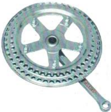
DO - 347 DOUBLE CHAINWHEEL & CRANK cottered 170 mm With & w/o Steel Guard Teeth = 38 - 48 / 40 - 48 / 42 - 52 For Chain = 1/2" x 3/32" BCP / BLACK Powder Coated
