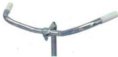
DO - 717 FRENCH Type BCP For Caliper Brake with PVC White Finger Type Grips Stem Size = 165 mm x 16 G Dia = 22.22 mm BCP
