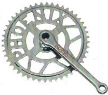
DO - 344 PHOENIX CUT Cottered Teeth = 44 / 46 / 48 Rounded Crank Size = 6-1/2" / 6-3/4" / 7" For Chain = 1/2" x 1/8"
