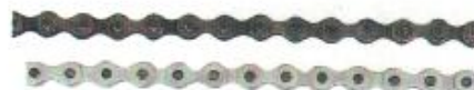
DO - 326 Bicycle Chain 1/2" x 1/8" or 1/2" x 3/32 Length = 66 to 116 Links Black / Golden Colour Breaking Load Min. 820 Kgs
